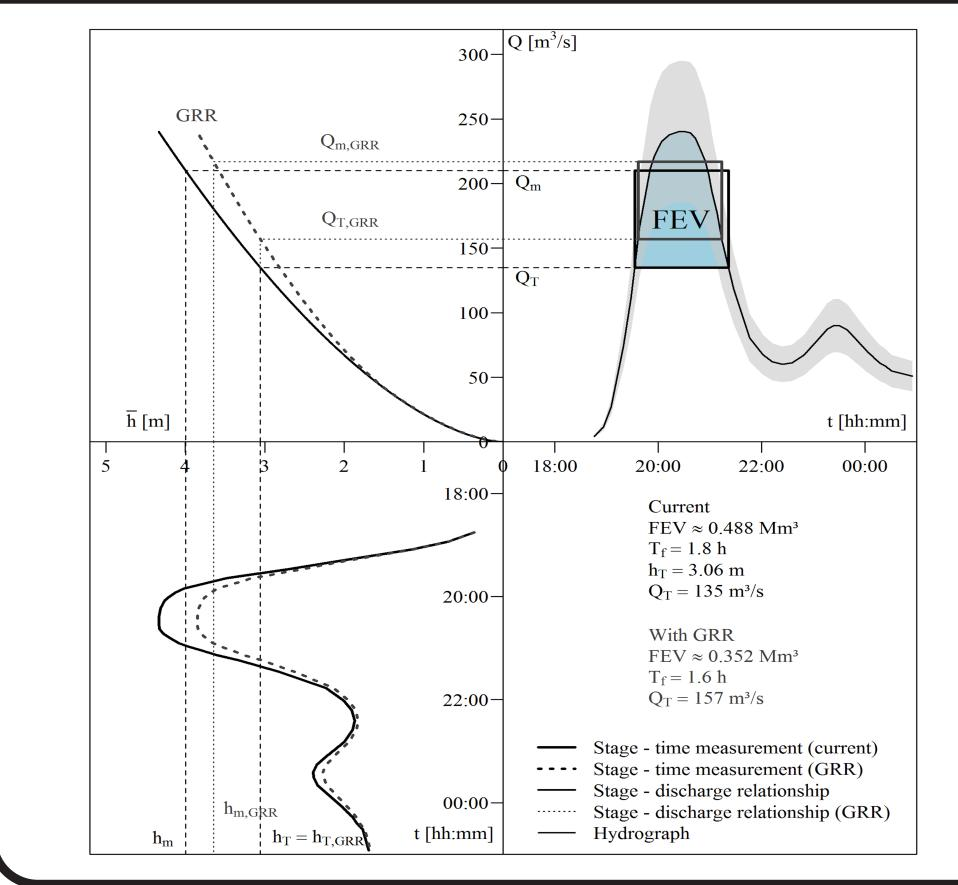
An alternative to raising flood walls: giving room to the river (GRR) increases the river width in order to increase the discharge capacity for a similar water depth.
